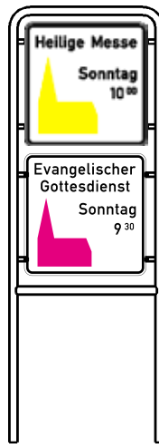
Standrohr-Ø 60,3/2,0 mm 2 x 750/750 mm
